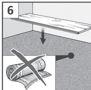
No offsets, steps or similar unevenness must be present. Construction rubble such as plaster residue or similar must be removed completely. Cracks in the ground must also be considered as critical. In order to assert full claims for damages, the provisions of ATV DIN 18365 and § 4 para. 3 VOB/B must be observed.
