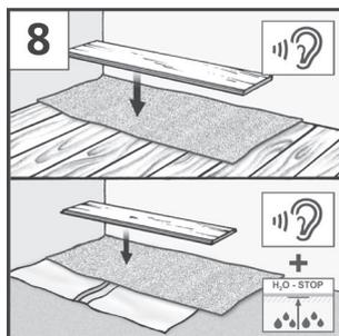
Lamination flooring is installed under "floating" conditions and may not be glued, screwed, nailed, or in any other fashion fixed to the floor! The placement of very heavy objects, such as fitted kitchens, also has a fixing effect. It is recommended to install fitted kitchens and cupboards before laying and to lay laminate floor only up to behind the plinth panel. In the event of failure to comply with these requirements any claims for damages shall be excluded [5]!
