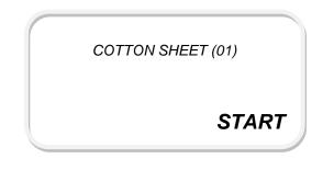
About roller ironers, tapping on the START icon the heating system starts.
