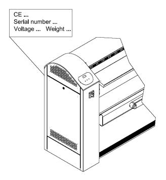
If this label is damaged, removed or absent, the machine cannot be identified; installation and maintenance operations become difficult and the warranty conditions expire automatically.
