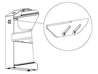
Unscrew the screw on both machine sides, position the table with the wished inclination and screw again the screws on both ironer sides.
