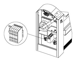
Following the kind of supply written on the serial number label, connect the cables to the terminal using a screwdriver:
