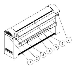
Point 1 identifies the ironer electric board access door. It can be opened using the plastic key supplied with the ironer documents. Only specialized and qualified technician may access to the electric board.
