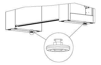
Check that the floor can support the machine weight indicated in the attached technical data sheet. The machine loading can be consider completely static.
