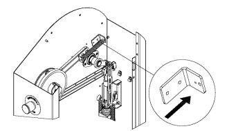
To take away the chest from the roller, pull up the bracket (the same in the above picture) so that the chest lifts and frees the limb, or the cloth, blocked into the ironer.
