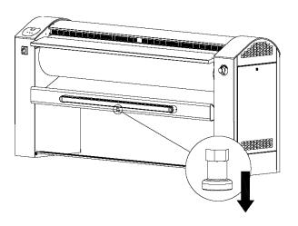
When the emergency is finished, free the bar pulling the spring pin to the bottom; it must be pulled until the anti-panic bar come back to its original position (see above picture).
