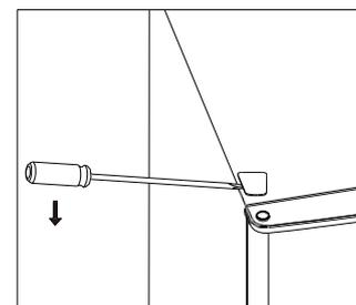
3. Move the core cover from left side to right side. And then lift the upper door and place it on a padded surface to prevent it from scratching.
