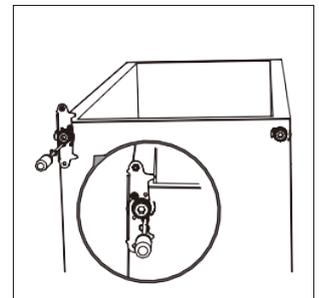
11. Place the door back on. Ensure the door is aligned horizontally and vertically so that the seals are closed on all sides before finally tightening the top hinge.
