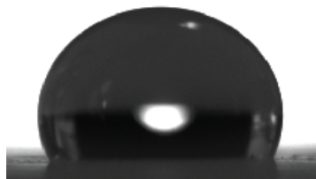
Water droplet on painted surface with SurfaPore Aqua X Additive+paint Contact angle: 126°
