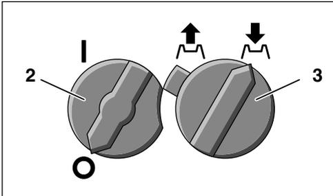
The rotational direction switch **3** must be turned to the right. The feed intake **1** must be empty.
