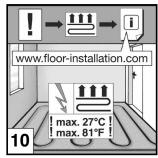
**Preparation:** Please store the packets 48 hours prior to installation under the same climatic conditions (temperature and moisture) as the actual installation process [1]. Important pre-condition for proper fitting and long-term durability of the laminated flooring is a room temperature of  $15 - 30^{\circ}$ C and a relative humidity of around  $40 - 70^{\circ}$ .
